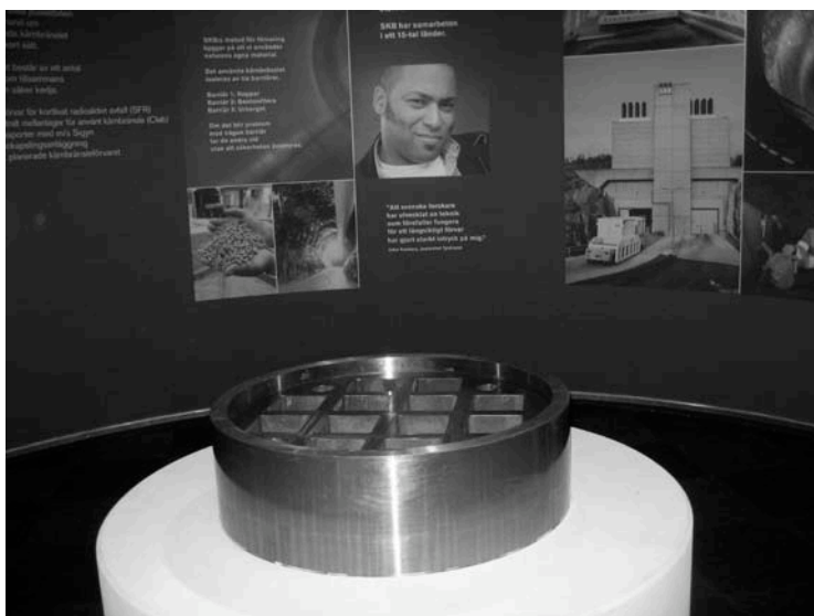
Figure 2. A section of a full-scale copper canister
