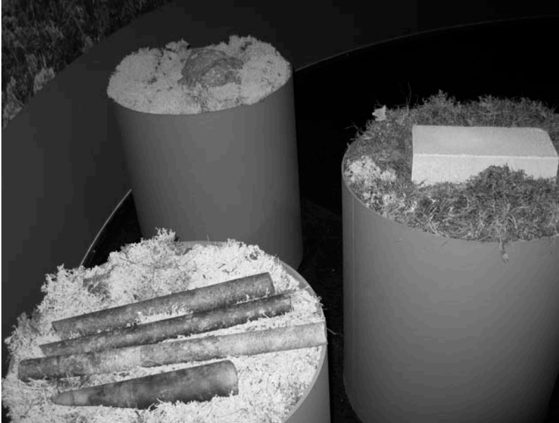
Figure 3. Three materials exposed: the bedrock, the betonite and the copper
